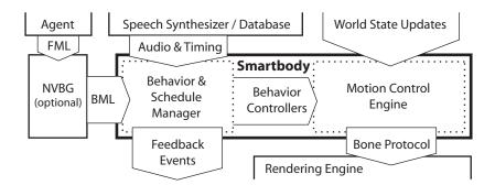
Figure 2: SmartBody processes BML, speech data, and world state to generate animation.
