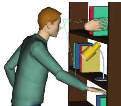
Figure 4: The polygonal line joining the character’s hand to the target hand represents the trajectory of the wrist joint for a valid collision-free motion.
