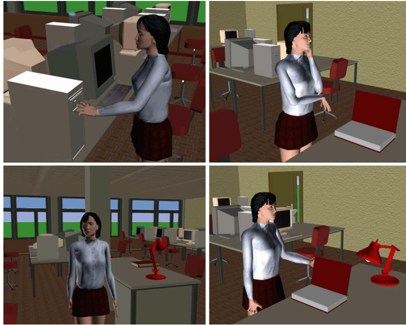
Figure 8.8 – Some snapshots of a simulation with ACE inside the virtual lab. Lisp plans are used to follow a simple storyboard, and orders from the Lisp behavioral module are sent through TCP/IP to control the actor in ACE. In parallel with the Lisp control, a Python thread runs to control the actor’s idle state.
