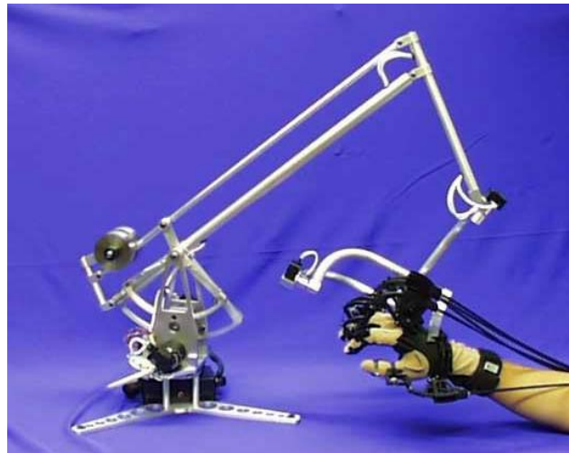
Figure 2.7 – The Cyber Force system from Virtual Technologies. Note that the external mechanical white arm, which provides the force feedback for the hand, can be also used to track the position and orientation of the hand. Force feedback at the finger level is provided by the small black exoskeleton mounted on top of the glove.
