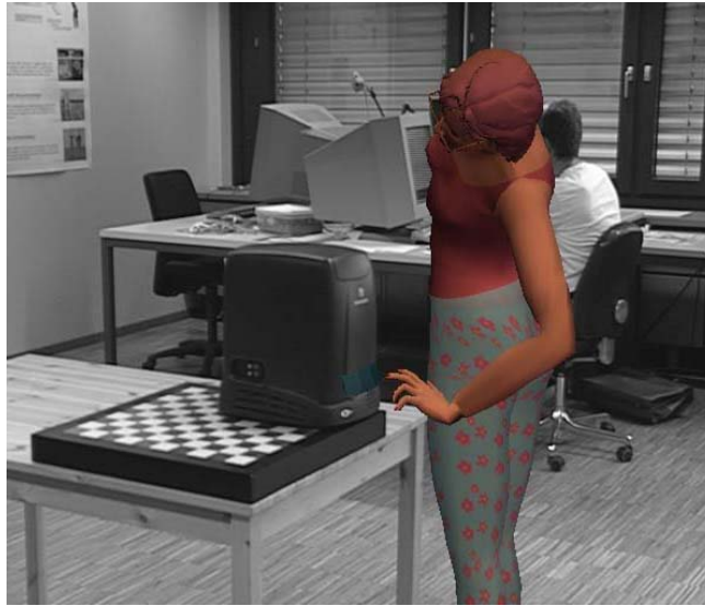
Figure 8.12 – An actor interacting with a smart object in an augmented reality environment. The computer and the background scenario are real. A virtual CD drawer was put in a lower position, to be tested as a design change in the computer. The virtual actor can interact with the added virtual part, giving a feedback for the design change. Such framework focuses simulation-based design of objects.
