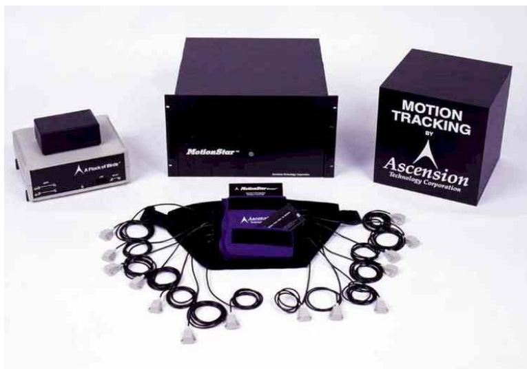
Figure 2.5 – Motion Star system of Ascension Technologies Corporation. The black box on the right is the emitter of the magnetic field. Sensors can be placed anywhere in the surrounding space and they will capture the position and orientation in space, relative to the emitter. The main drawbacks of such magnetic systems are the interference caused by metallic objects, and the limited work volume size.
