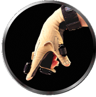
Figure 2.6 – The Cyber Touch glove of Virtual Technologies. This data glove uses fiber optics to measure fingers flexion. Tactile sensors are mounted in each finger and in the palm, in order to provide vibration sensations.
