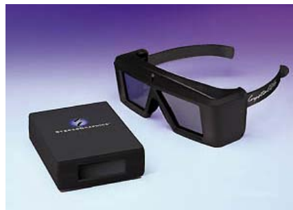
Figure 2.8 – The Shutter Glasses of Stereographics. The image shows the glasses and the infrared synchronizer that, when connected to the computer, synchronizes which lens of the glasses need to block the light, in order to let each eye see the correct image. The graphical software is required to generate different images for each eye in a sequential form.
