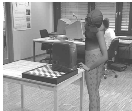
Figure 5 a, b: A Virtual Human testing a virtual CD-ROM driver from different distances. The driver is placed lower. In these images a virtual model of the CD-ROM is placed in a lower position in the O2, like in the Figure 2.
