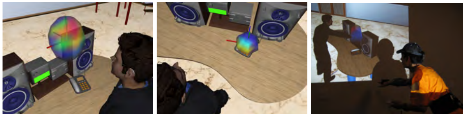
Fig. 9. The local coverage visualizer can be interactively placed over a small ROI during the motion modeling phase, enabling the user to instantly visualize the current motion cluster coverage at important locations. The user can then easily further improve the cluster as needed. The right-most image shows the user interactively placing the local coverage visualizer close to the control panel of the sound system to inspect the cluster coverage in those specific regions.
