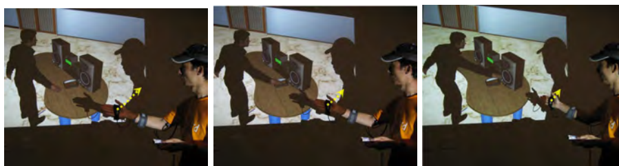
Fig. 7. This example interface allows the user to easily scroll through captured motions, crop out unwanted frames, and most importantly mark stroke frames to be parameterized. This image shows the user inspecting one motion segment with a simple hand movement.
