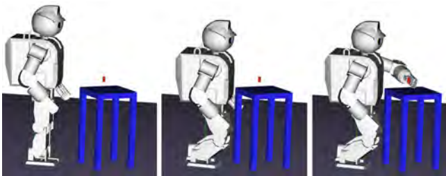
Fig. 1. Example of a simple reaching task which is only solvable after the robot performs a few stepping motions and body adjustments.
