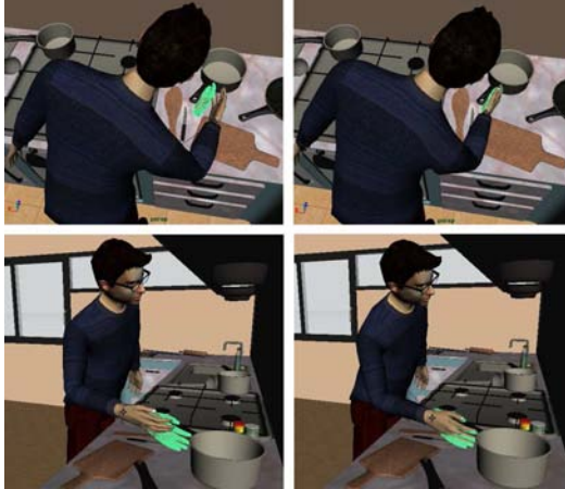
Figure 4: The closest configuration in the roadmap in relation to the target hand (left column), and after the probabilistic IK process (right column).
